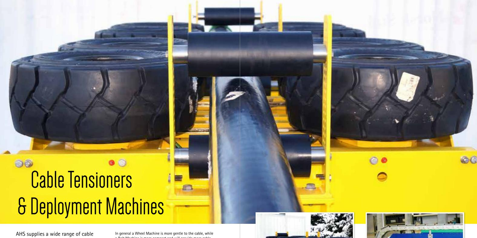
AHS supplies a wide range of cable tensioners, cable transporters and deployment machines for power, communication and sensor cables. These are either wheel based or belt based, often referred to as linear cable engines and tracked engines. We call them Wheel Machines and Belt Machines.
